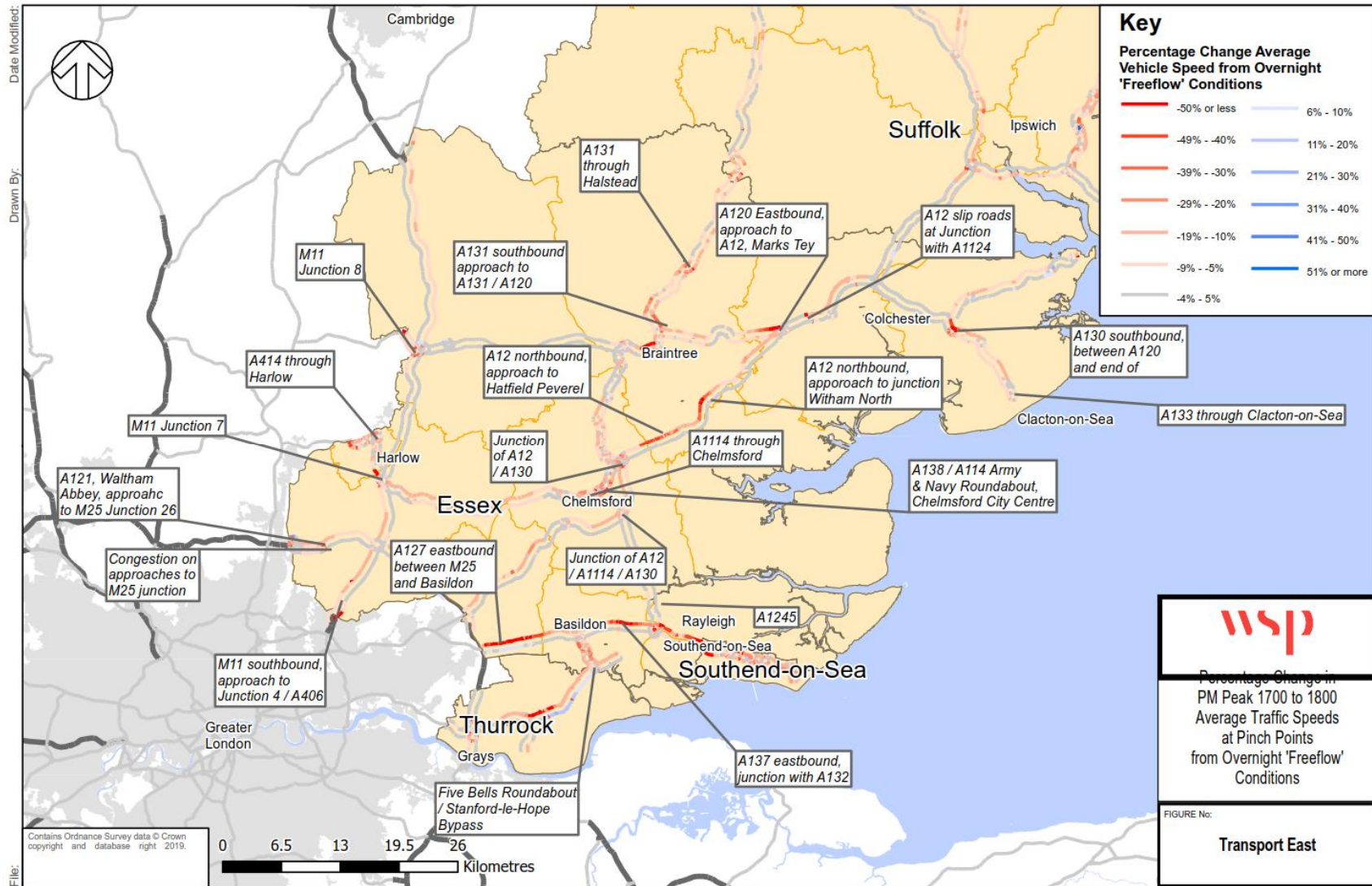
Figure 5-25 – Change in median vehicle speed between overnight (“free flow conditions”) and PM Peak – Essex
